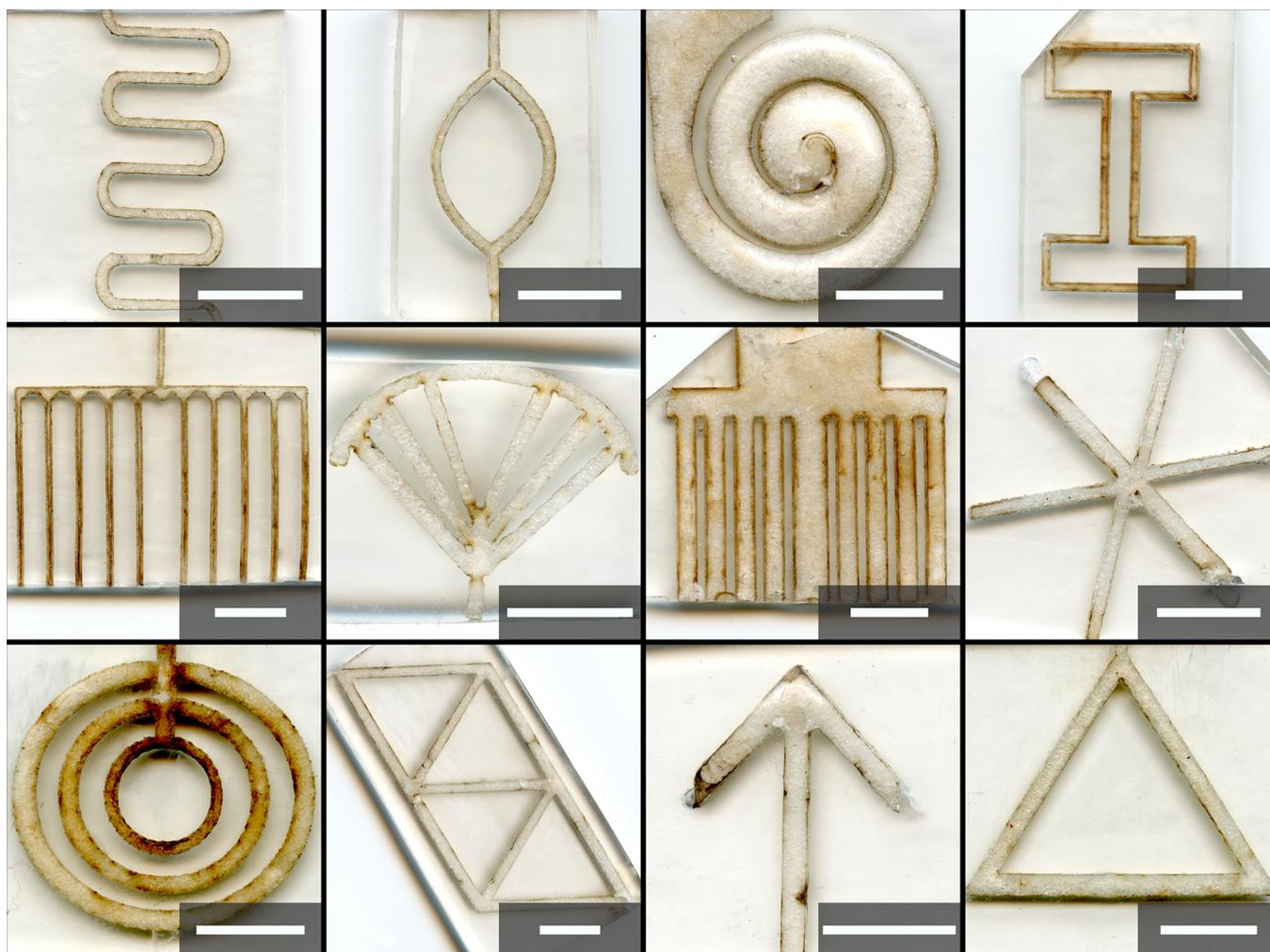
**Figure 2.** Array of accessible geometries for frontal polymerization in vascular structures. Features investigated included curvature and branching. All microchannels shown here were fabricated using the catalyzed depolymerization of laser-cut polylactide sheets, approximately  $600\ \mu\text{m}$  in thickness. Channel widths range from 1 to 2 mm. Propagation through the entire sample with one initiation was observed in most cases. All scale bars are 1 cm.
